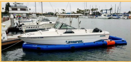
Fab Dock in-water dry docking system that was used in the County's 6-month trial with a Sea Scout vessel
